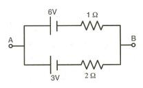
**36.** Two batteries of different emfs and different internal resistances are connected as shown. The voltage across AB in volts is
